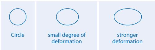
The Deformation Index is calculated as the relationship between the differences in size of the two meridians of the ellipsoid. The greater the difference between the two meridians, the greater the deformation.
