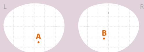
2. By repositioning the addition in the lens, both eyes experience the same accommodation support.
