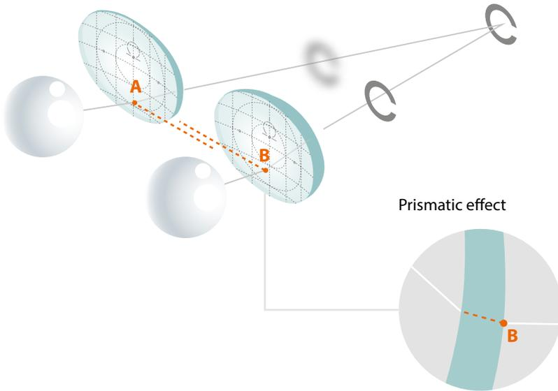
Due to different prismatic effects, the light rays pass through the lens at different positions for the right and left eye.
