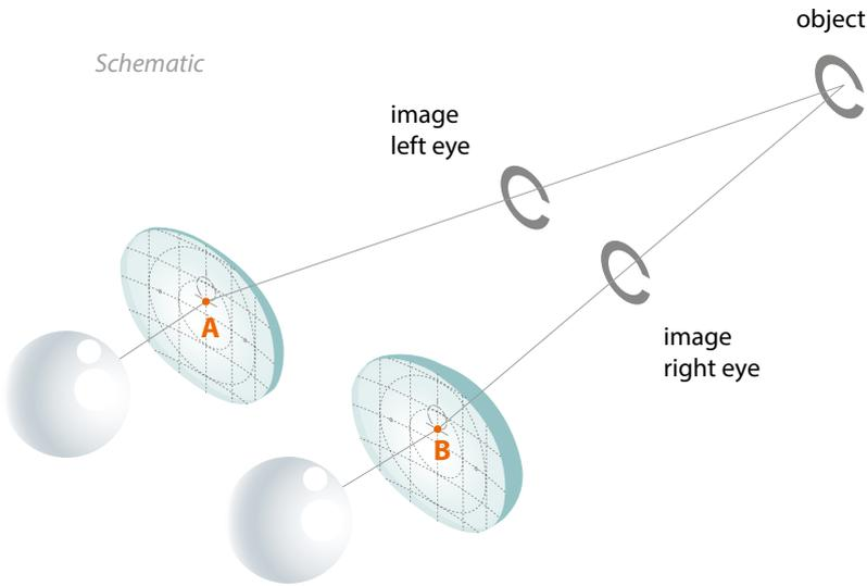
A and B: position where light ray passes through the lens
