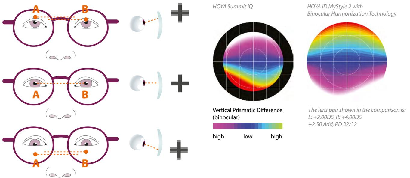
Figure 19: Comparison Vertical Prismatic Difference (binocular)
