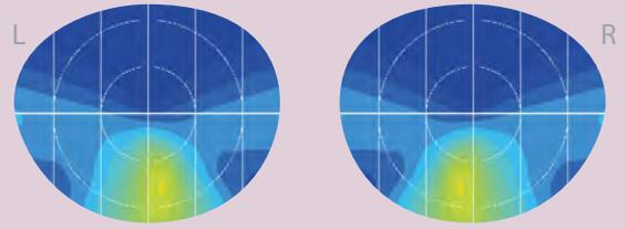
If both eyes are in the central position, light rays pass through the lens at the same point. Therefore, both eyes experience the same addition power.
