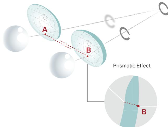
Due to different prismatic effects, are deviated at different rates for the right and left eye.
