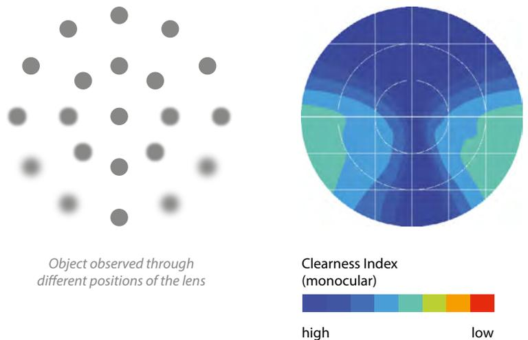
Figure 10: Principle of Clearness Index
